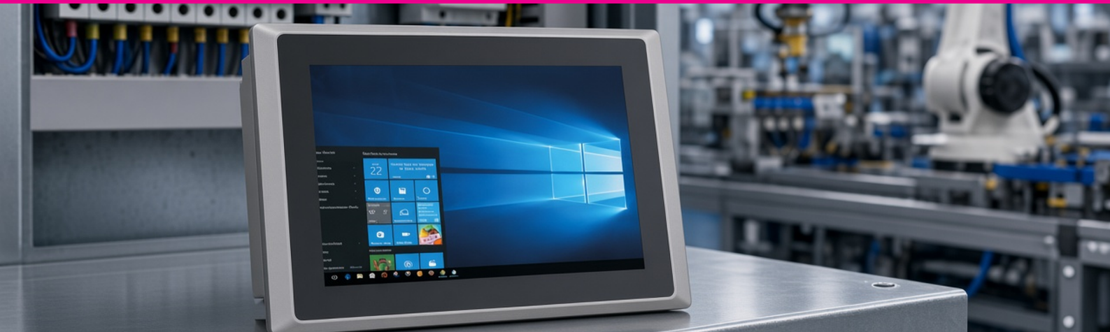
Fanless touch panel for industrial control – front IP65, dual LAN and dual serial.
